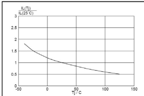
Fig.8. Normalised latching current  $I_L(T_j)/I_L(25^\circ C)$ ,
