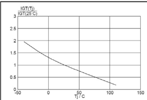
Fig.7. Normalised gate trigger current
