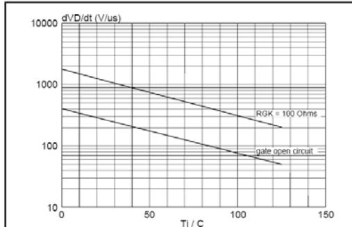
Fig.12. Typical, critical rate of rise of off-state voltage,
