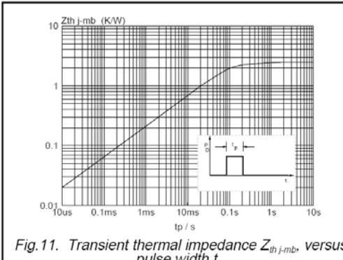
Fig.11. Transient thermal impedance  $Z_{th\ j\ mb}$ , versus
