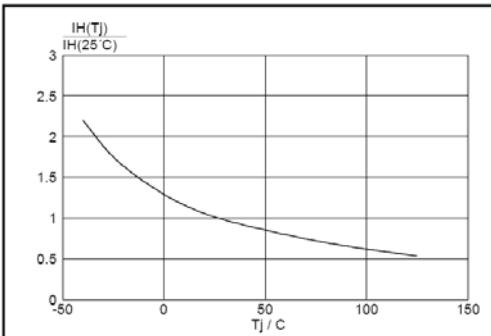
Fig.9. Normalised holding current  $I_H(T_j)/I_H(25^\circ C)$ ,
