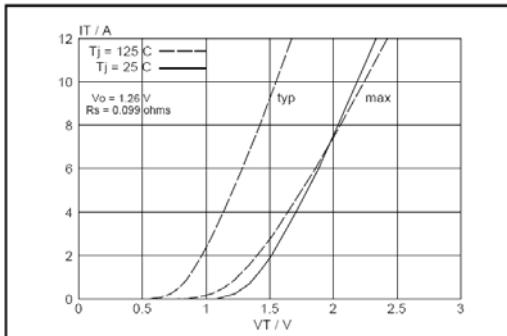
Fig.10. Typical and maximum on-state characteristic.
